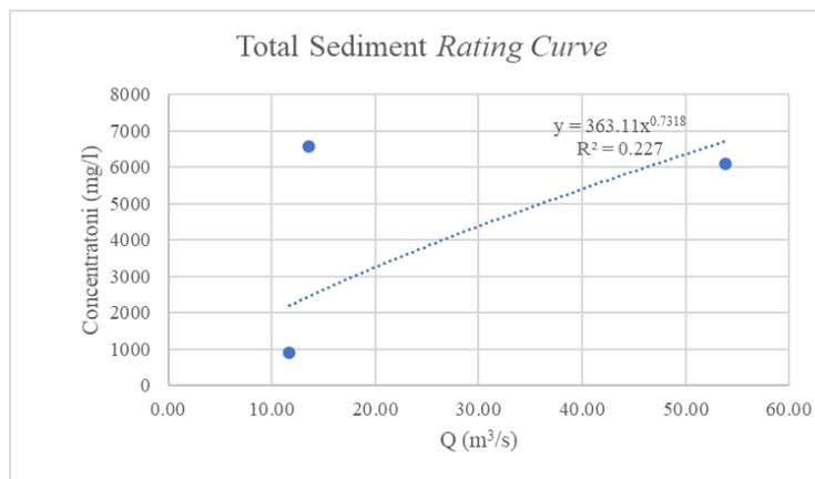
**Figure 10.** Total Sediment Rating Curve
