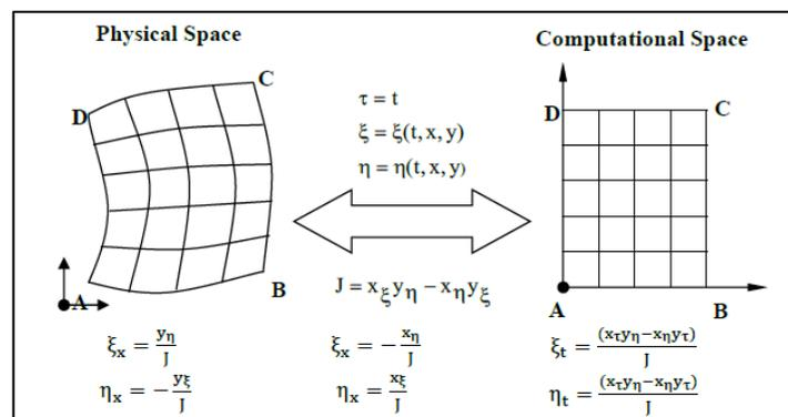
**Figure 1.** Generalized Curvilinear Coordinate Transformations
