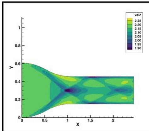
**Figure 8.** Contour of velocity flow for 10 seconds simulation
