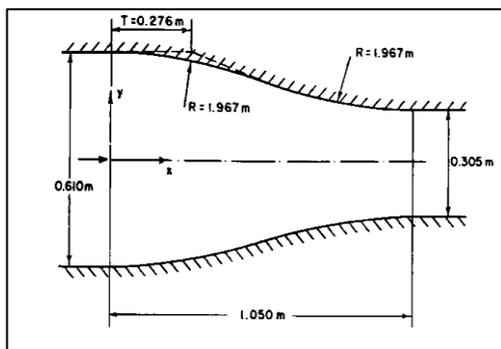
Figure 2. Profile Circular-arc
