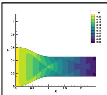
Figure 6. Contour of water depth for 10 seconds simulation
