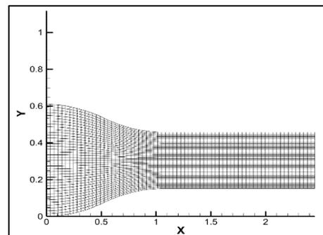
Figure 3. Curvilinear grids of Circular arc
