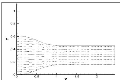
Figure 3. Flow vector pattern of circular-arc case
