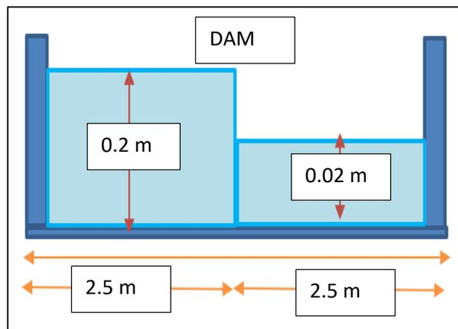
**Figure 8.** Dam break model
