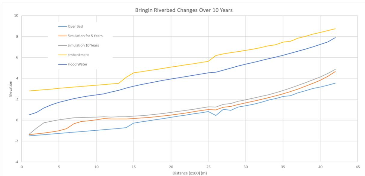
**Figure 2.** riverbed change with 10 years simulation using HEC-RAS
