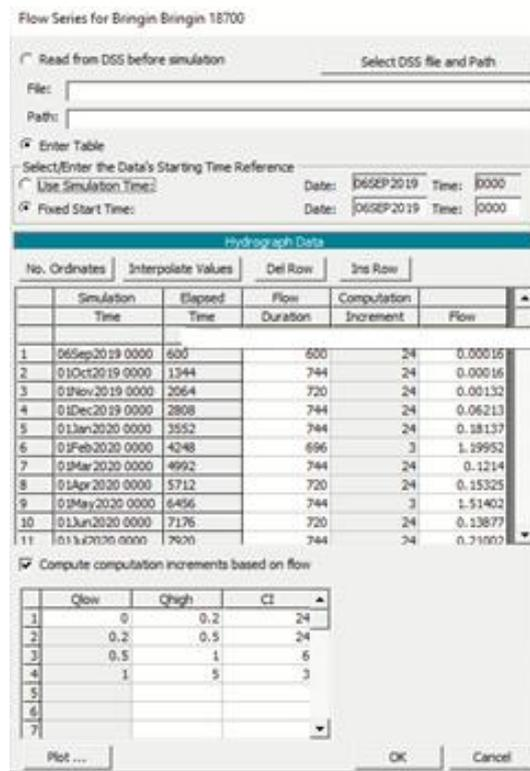
Figure 9. Flow Series (Upstream Boundary Condition)
