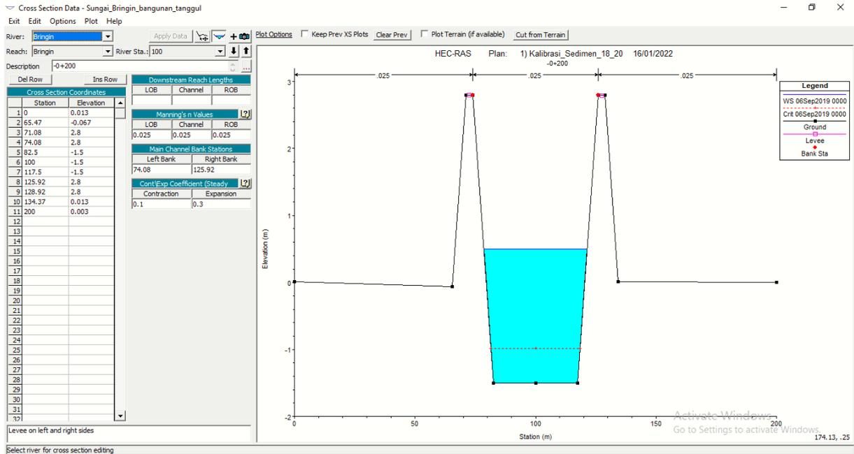
Figure 15. HEC-RAS display using flood control building
