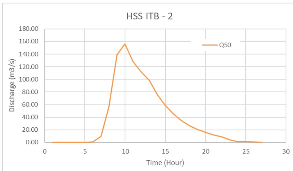
**Figure 14** flood hydrograph HSS ITB 2 Method
