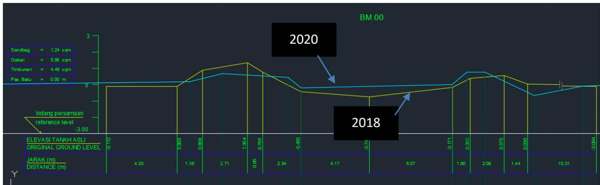
Figure 3. Comparison of the Bringin Riverbed in 2018 and 2020 at Sta 0+000
