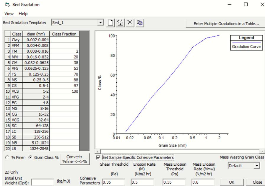
Figure 7. Bed Gradation at Point Location 1
