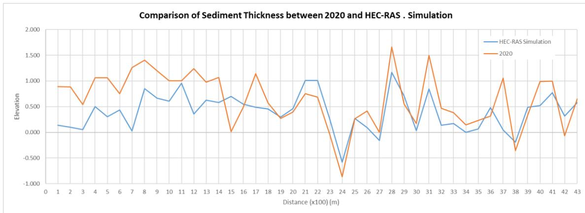
**Figure 13** Comparison of Sediment Thickness between 2020 and HEC-RAS Simulation
