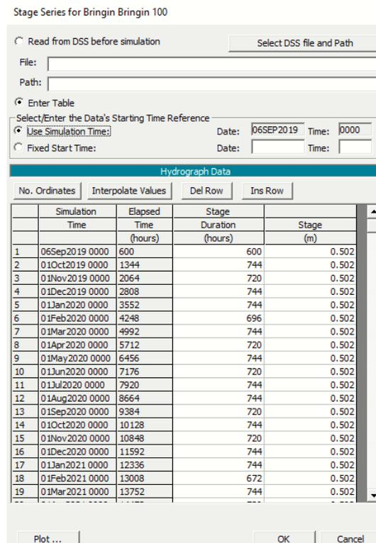
Figure 10. Stage Series (Downstream Boundary Condition)
