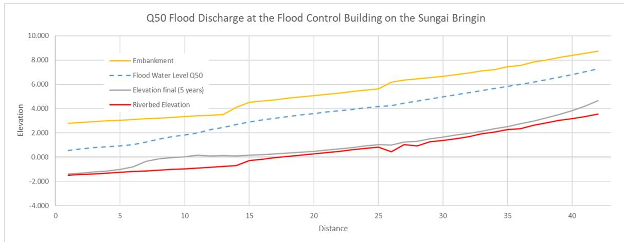
**Figure 1.** riverbed change with 5 years simulation using HEC-RAS
