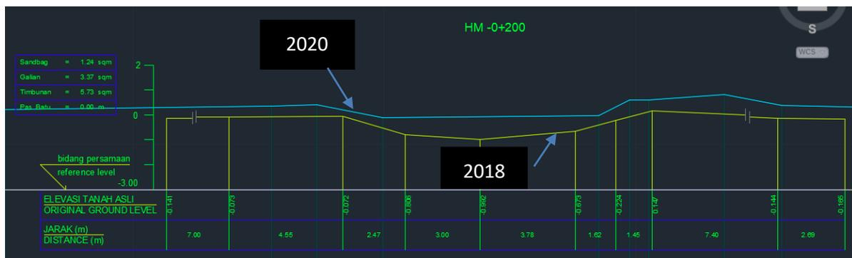
**Figure 2.** Comparison of the Bringin Riverbed in 2018 and 2020 at Sta -0+200
