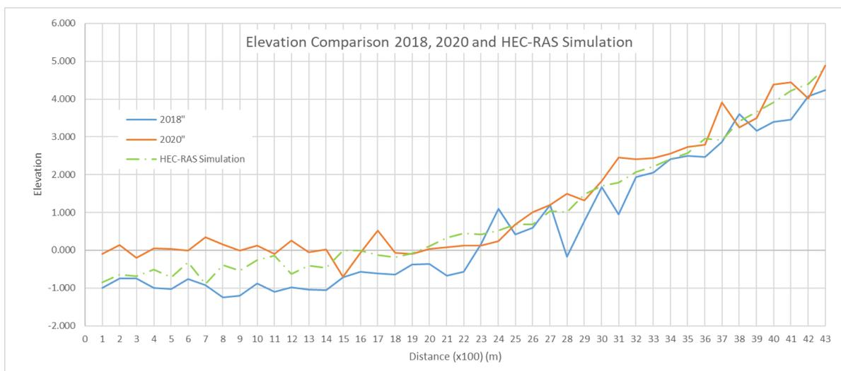
**Figure 12** elevation comparison between HEC-RAS simulation and geometry data
