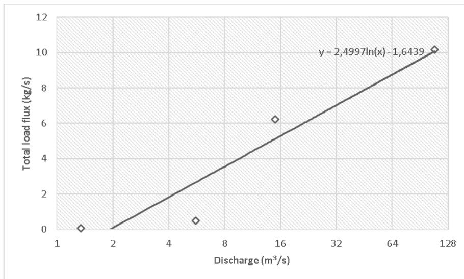
**Figure 5.** Relation between discharge and sediment rate of total load.
