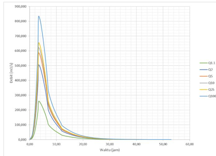
**Figure 2.** The flood hydrograph of the Nakayasu method.
