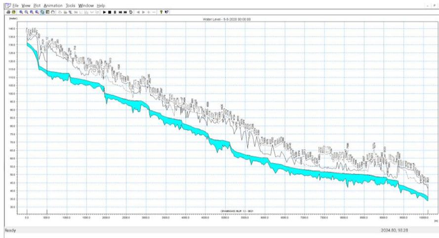
**Figure 4.** Simulation results for the 2-year return period discharge using the Nakayasu.
