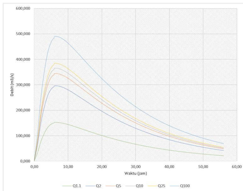
**Figure 3.** The flood hydrograph of the Snyder method.
