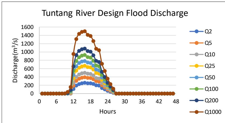
**Figure 10.** Tuntang River Design Flood Discharge
