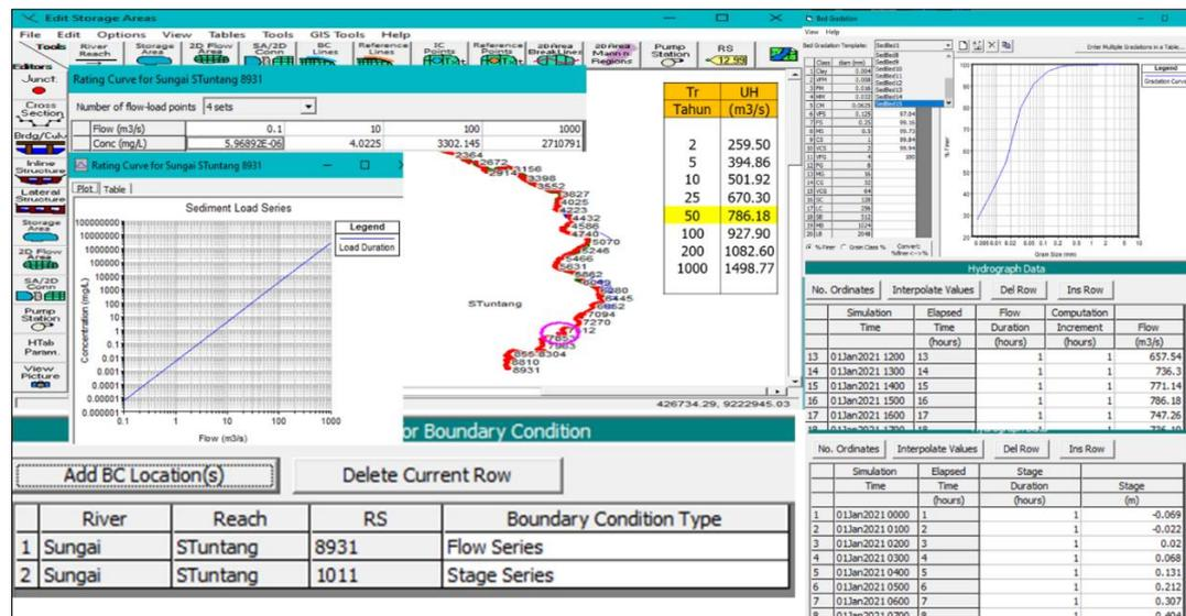
Figure 7. Boundary Condition Quasi Unsteady Flow 1D Q50 River Morphology
