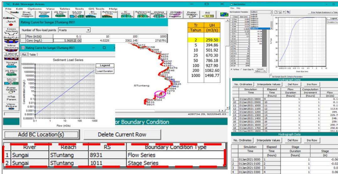
Figure 6. Boundary Condition Layout Quasi Unsteady Flow 1D Q2 River Morphology
