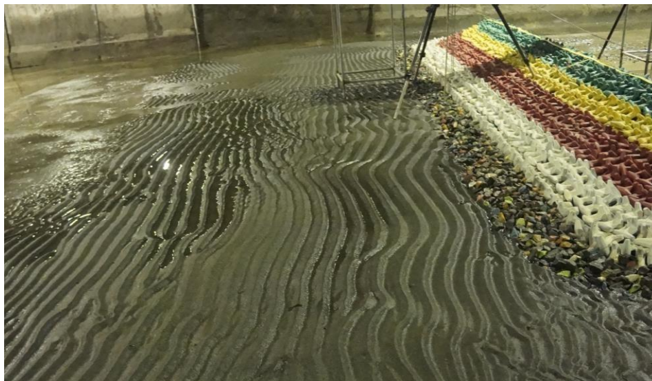
Figure 11. Sediment condition after loaded with daily waves simulation
